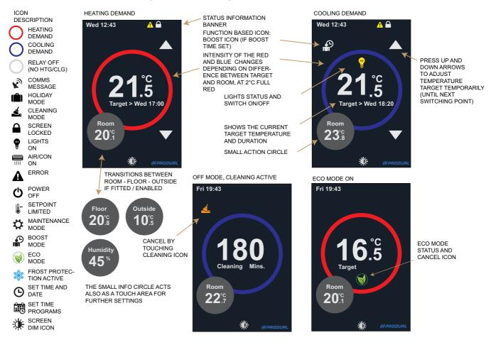
The TRT-P-1R room thermostat home screen has four touch sensitive areas that allow the thermostat settings to be changed.
